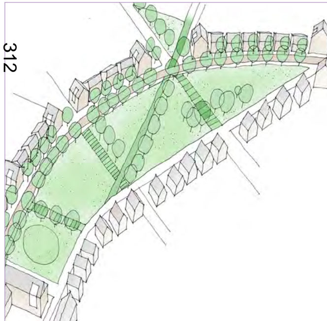
Sketch illustrating how buildings can successfully provide overlooking and enclosure to an open space.
